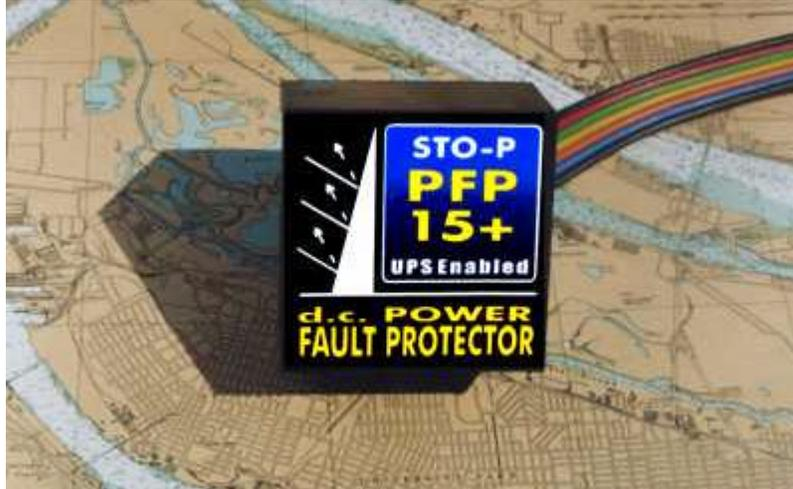
PFP15 Power Fault Protector is compact in size for tight installations. It is 'UPS enabled' with switching and charging controls but requires user supplied backup battery mounted externally. Provides a total of 15 amps of safe power to two separate outputs. The UPS output can supply up to 10 Amps of backup power.
