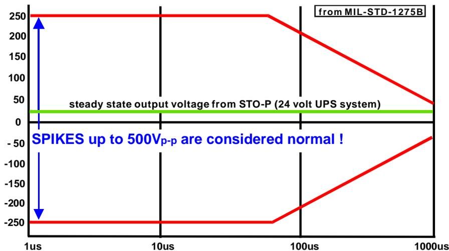
In vehicles, windscreen wiper motors, lamp flashers and ignition sparks are typical sources of spikes. In the marine environment, bilge pumps, relays and solenoids produce spikes capable of damaging semiconductors.
