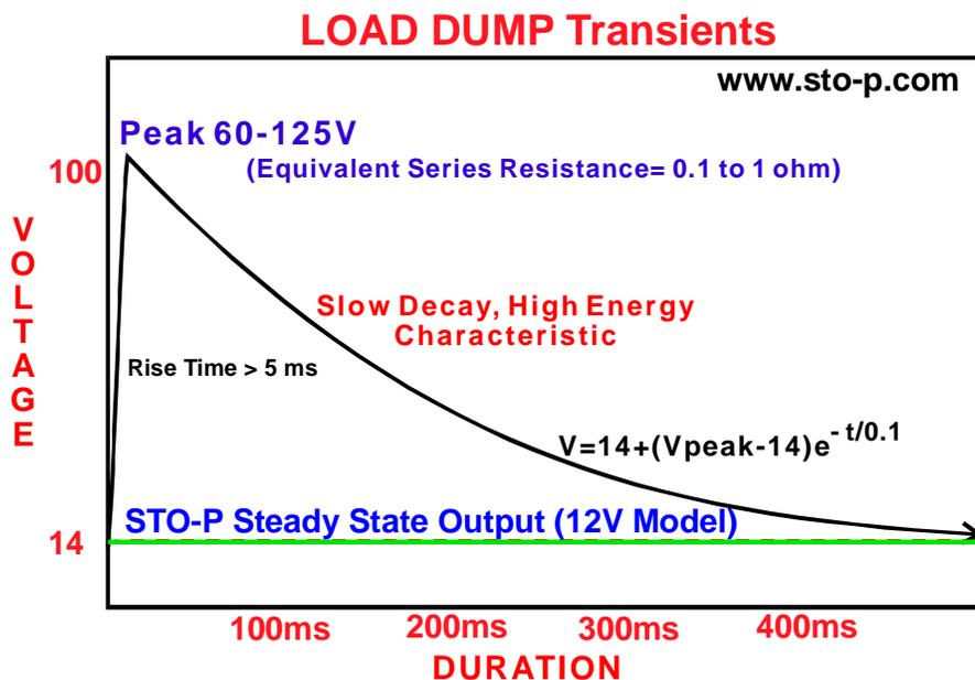
Destructive 'LOAD DUMP' transients occur when a battery is disconnected from the charging system during moderate or high charging rates. Load dump transients typically reach peak voltages of 60 to 125 volts in 12 volt systems with relatively slow rise times. Their duration usually exceeds several hundred ms and can extend out to 1 second or more depending on the characteristics of the charging system.
