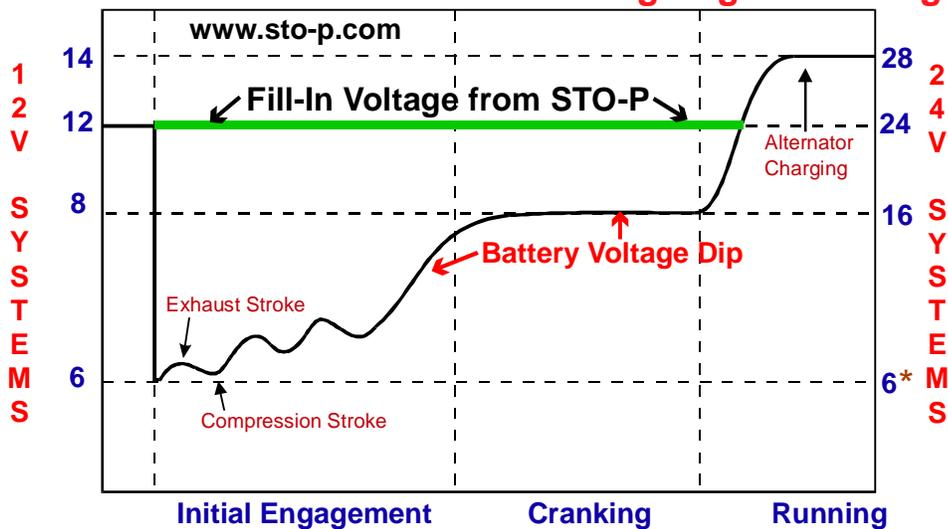
**Voltage levels for 12 Volt Systems shown on the Left and corresponding levels for 24 Volt Systems shown on the Right.**
